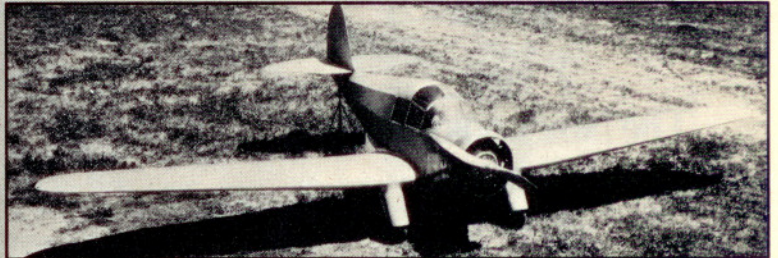
Aeronca Model LC Introduced in 1937 Two-place, side-by-side seating Low wing Warner Scarab Jr. radial engine
