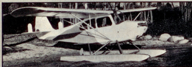
Aeronca Model 7AC (Champion) Introduced in 1945 Two-place, tandem seating Metal rib, high wing 65-hp Continental engine
