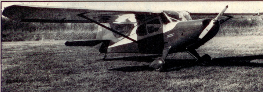
Aeronca Model 7AC (Champion) Introduced in 1945 Two-place, tandem seating Metal rib, high wing 65-hp Continental engine
