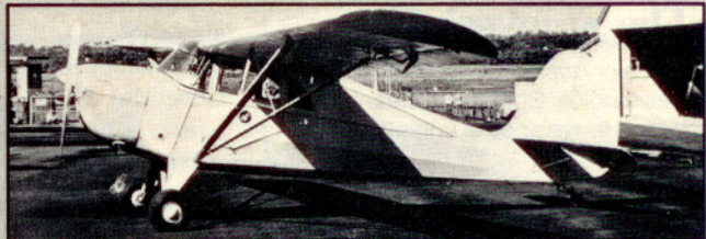
Aeronca Model 65CA (Super Chief) Introduced in 1940 Two-place, side-by-side seating High wing 65-hp Continental engine
