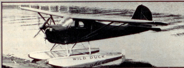
Aeronca Model K Introduced in 1936 Two-place, side-by-side seating Wing brace struts External front "Y" exhaust 40-hp, 42-hp or 45-hp Aeronca engine
